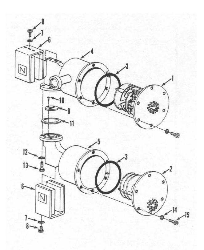
Figure 4-2 MS-40 Mass Spectrometer (Exploded View)
